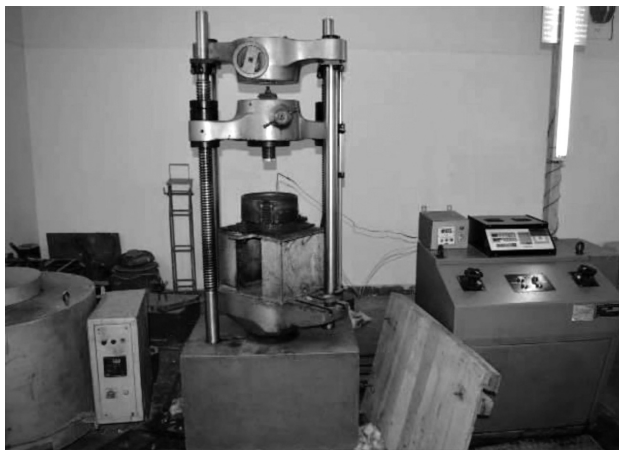
Figure 2: Modified universal testing machine for squeeze casting
