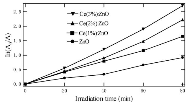
**Figure 6:**  $A_0/A$  as a function of irradiation time for methyl blue photodegradation using Ce:ZnO as the photocatalyst
