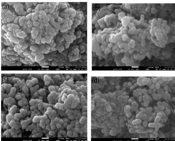
**Figure 3:** FSEM images of Ce-doped ZnO, Ce concentrations of: a) 0 %, b) 1 %, c) 2 % and d) 3 %
