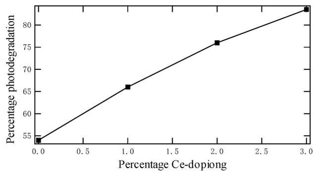
**Figure 5:** Percentage of photodegradation vs Ce-doping after 60 min of UV irradiation
