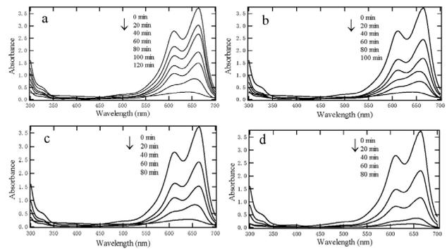
**Figure 4:** Absorbance changes of methyl blue with UV irradiation time for: a) pure ZnO, b) 1 % Ce, c) 2 % Ce and d) 3 % Ce:ZnO nanoparticles as the photocatalysts
