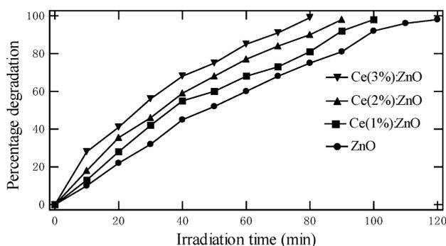
**Figure 7:** Percentage of photoabsorbance of methylene blue with Ce-doped ZnO samples vs UV irradiation time
