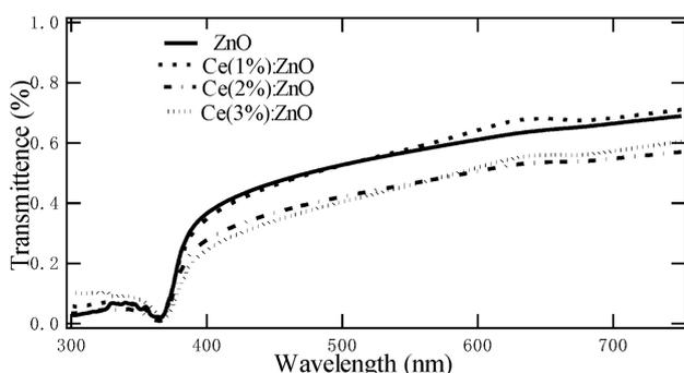
Figure 1: Transmittance spectra of the Ce:ZnO nanoparticles
