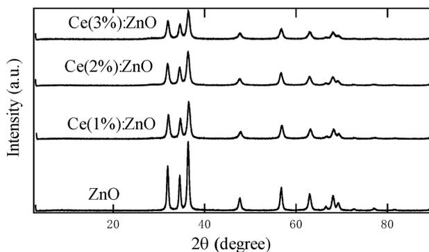
Figure 2: XRD patterns of the Ce:ZnO nanoparticles with Ce concentrations of (0, 1, 2 and 3) %
