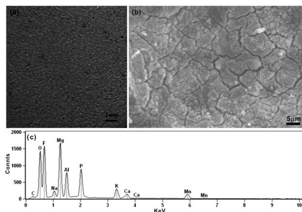
**Figure 1:** a) Macromorphology, b) SEM image and c) EDS spectrum of a conversion coating deposited on AZ91D magnesium alloy
