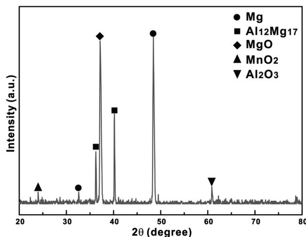
**Figure 3:** XRD pattern of a conversion coating deposited on AZ91D magnesium alloy
