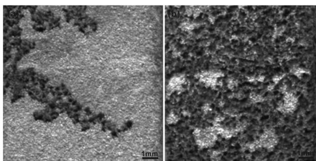
**Figure 4:** Corrosion morphologies of the samples: a) with a conversion coating and b) without conversion treatment
