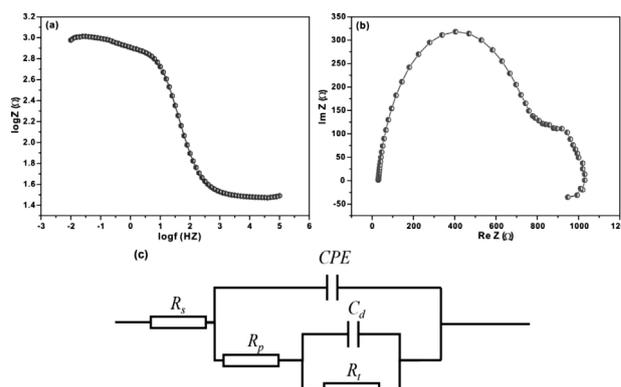
**Figure 5:** a) EIS Bode plot and b) Nyquist plot of the converted AZ91D magnesium alloy in a 5 w/% NaCl solution, and c) the equivalent circuit for fitting the EIS data
