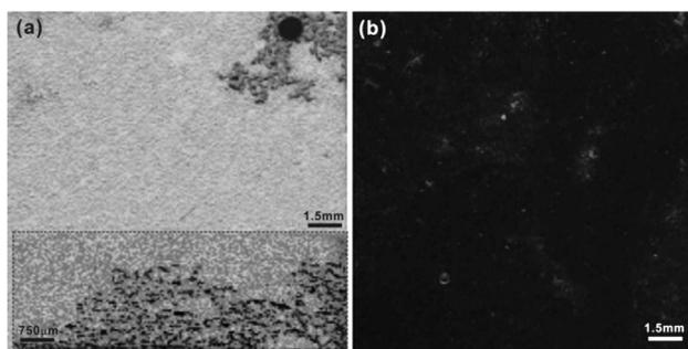
**Figure 7:** Corrosion morphologies of the sample with a conversion coating after immersion in a solution of 3.5 w% NaCl for two days (upper side) and five days (lower side) a) and the sample with an organic coating applied onto the conversion substrate under a neutral salt spray of 3.5 w% NaCl for five days b)
