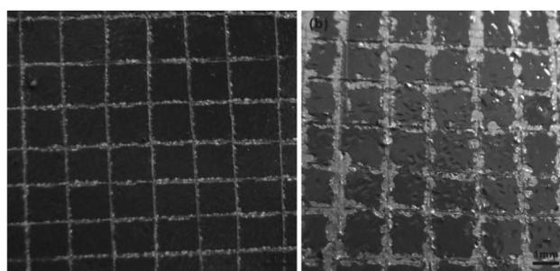
**Figure 6:** Surface morphologies of the scratched patterns on the organic coatings on the surfaces of AZ91D magnesium alloy samples a) with and b) without a conversion coating
