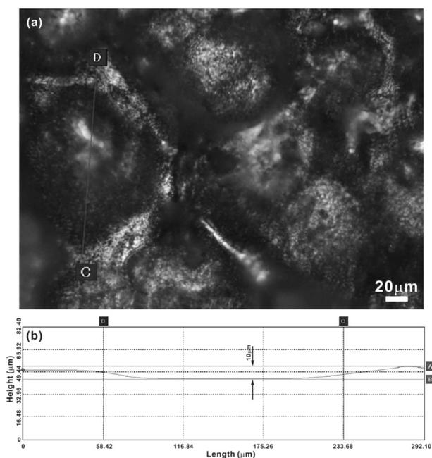
**Figure 2:** a) DM image of a conversion coating and b) the corresponding line scanning profile from point C to point D
