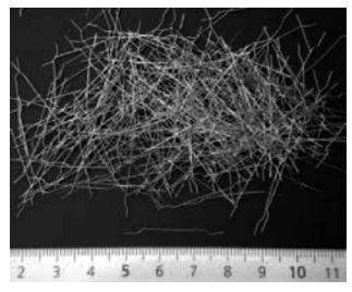
Figure 1: Steel fibers
