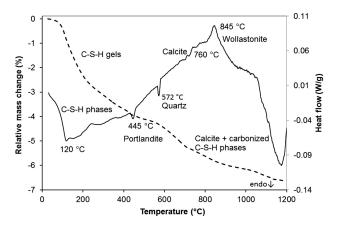
Figure 3: DSC and TG curves of the studied HPFRC
