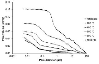
Figure 2: Cumulative pore-size distribution
