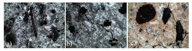
Figure 5: Optical-microscopy images of HPFRC: a) reference sample, b) sample exposed to 600 °C, c) sample exposed to 1000 °C
