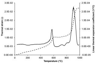
Figure 4: Thermal strain and linear thermal expansion coefficient of the studied HPFRC
