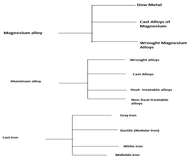
Figure 2: Materials classification: Mg alloy classification, Al alloy classification, cast iron classification
