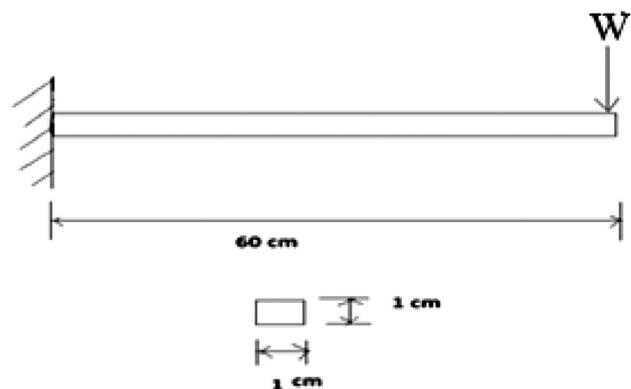
**Figure 5:** CAD model for static load condition
