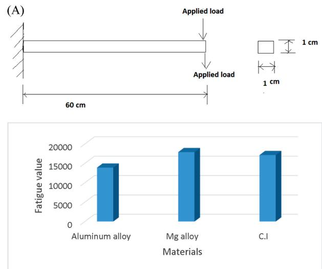
**Figure 6:** Fatigue analysis: a) CAD-model for fatigue load condition, b) fatigue value for Mg, Al and cast iron
