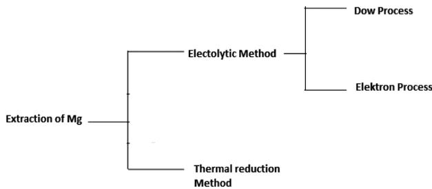
Figure 1: Extraction methods for Mg alloy
