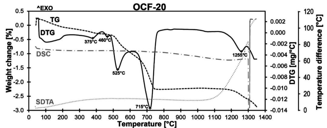
Figure 8: DTA/TG and DSC analysis of test sample OCF-20
