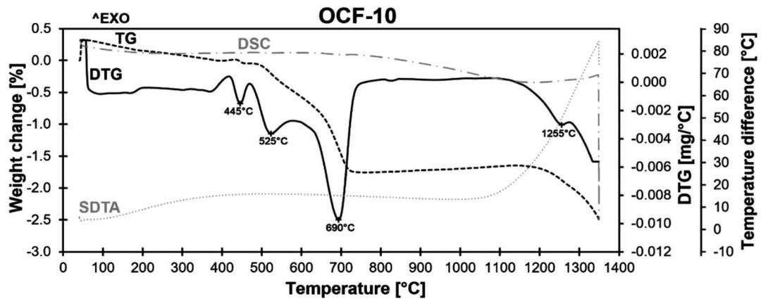
Figure 7: DTA/TG and DSC analysis of test sample OCF-10
