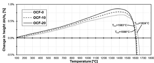
**Figure 3:** Determination of refractoriness under load of the mixtures with different amounts of fly ash
