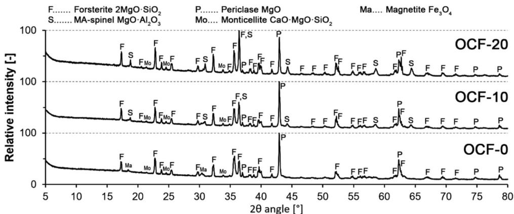
Figure 5: X-ray diffraction patterns of all the mixtures with different amounts of fly ash
