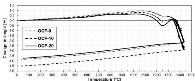
**Figure 2:** Thermal dilatometric analysis of the mixtures with different amounts of fly ash
