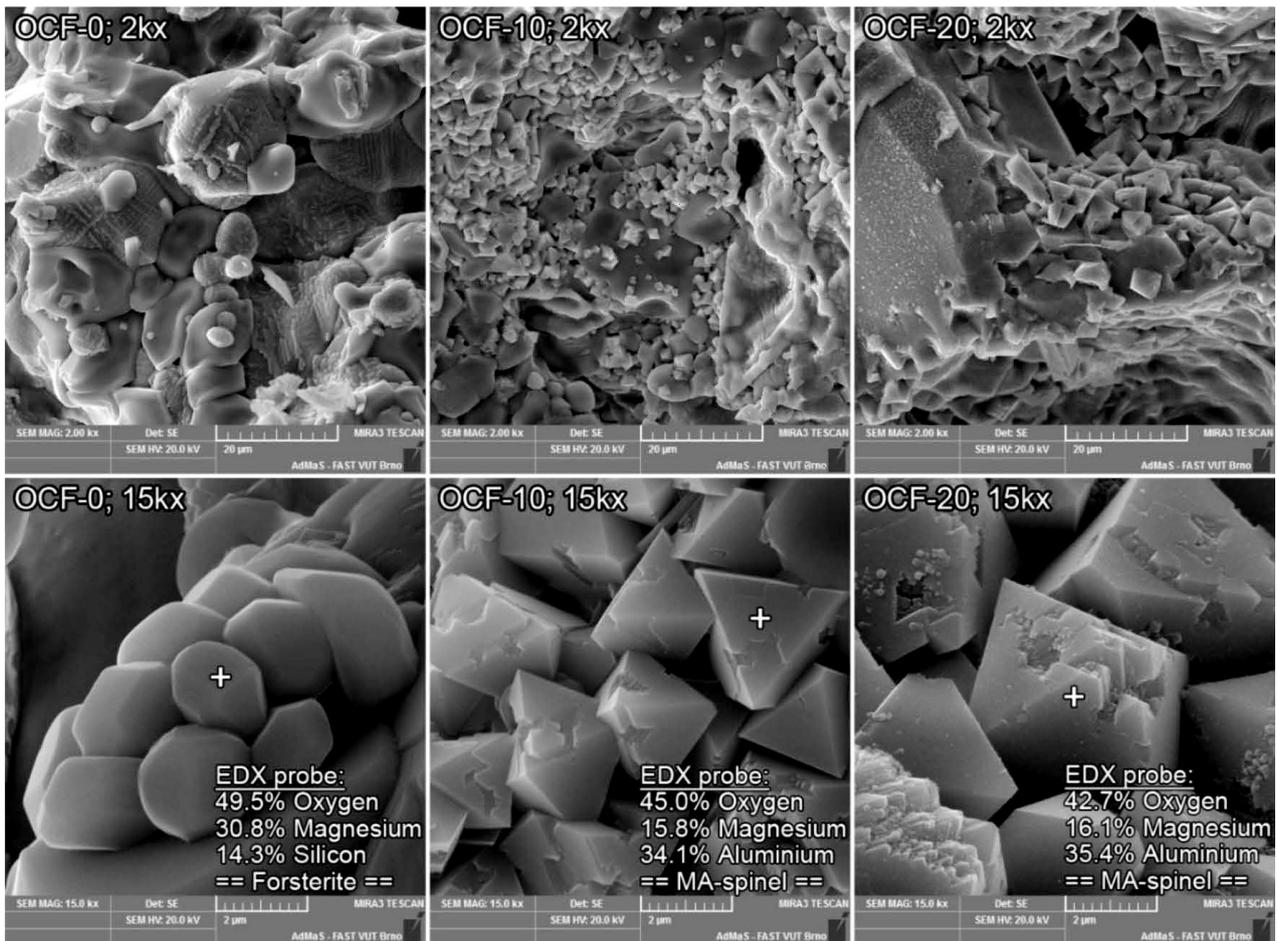
Figure 4: SEM of different mixtures with magnifications of 2000x (top) and 15000x (bottom)
