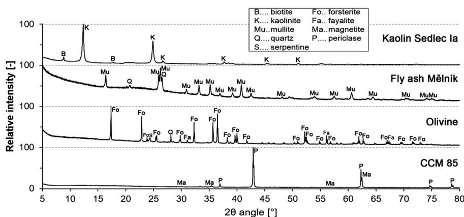
**Figure 1:** XRD of the used raw materials without heat treatment
