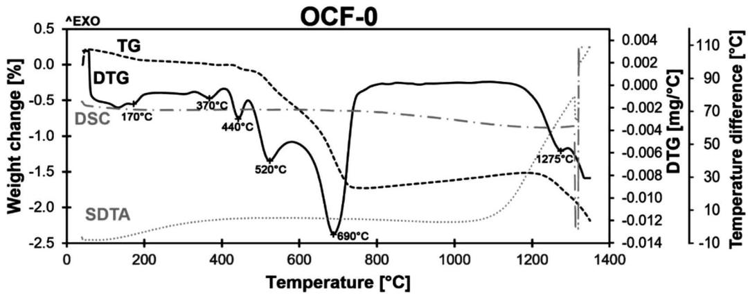
Figure 6: DTA/TG and DSC analysis of test sample OCF-0
