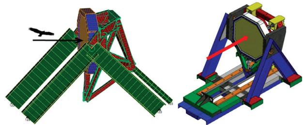
**Figure 4:** Experimental-stand configuration for a perpendicular impact<sup>7,8</sup>
