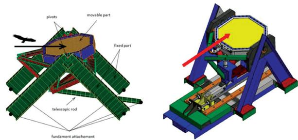
**Figure 3:** Experimental-stand configuration for a low-angle impact<sup>7,8</sup>
