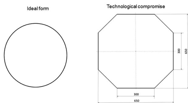
**Figure 2:** Optimized specimen form
