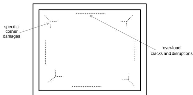
**Figure 1:** Typical non-regular flaws of a standard square specimen
