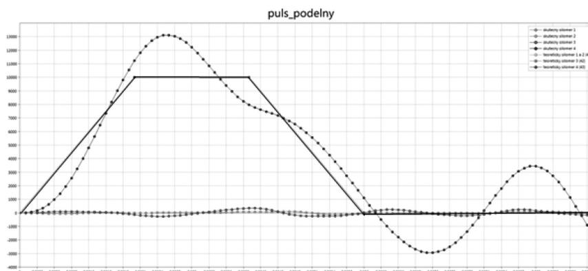
Figure 5: Example of virtual-load-cell records for a specimen-plane applied force<sup>7</sup>
