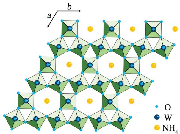
Figure 4: Crystal structure of the as-prepared  $(\text{NH}_4)_x\text{WO}_3$  sample
