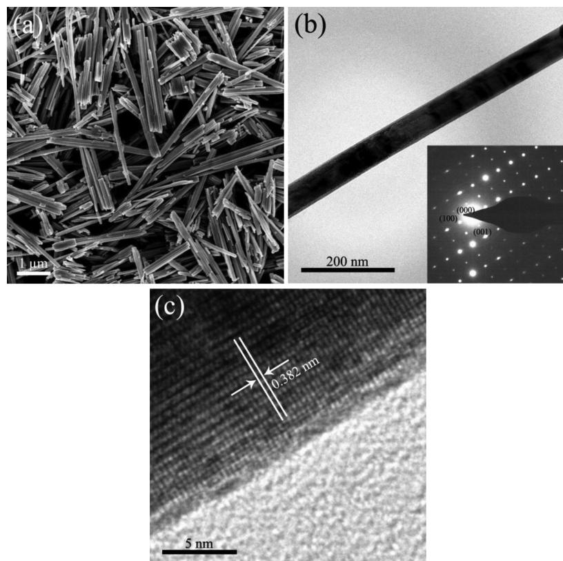
**Figure 2:** a) SEM image, b) TEM image and c) HRTEM image of the as-prepared  $(\text{NH}_4)_x\text{WO}_3$  sample. The inset shows the corresponding SAED pattern (b)
