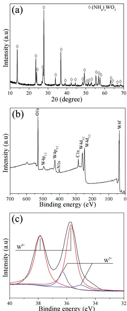
**Figure 1:** a) XRD pattern, b) full-range XPS spectra and c) W4f core-level XPS spectra of the as-prepared  $(\text{NH}_4)_x\text{WO}_3$  sample
