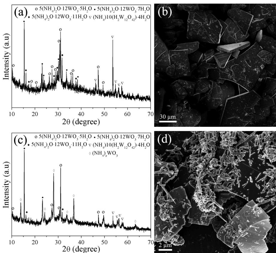
**Figure 3:** XRD pattern and SEM image of the products after reaction times of: 2 h (a, b) and 6 h (c, d), respectively
