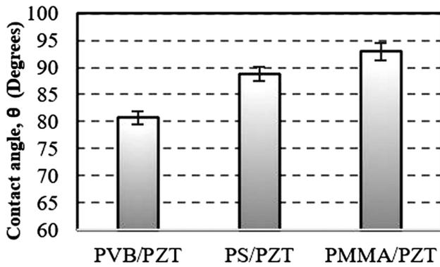
Figure 4: Mean contact angle of water droplet on three different PZT polymer surfaces
