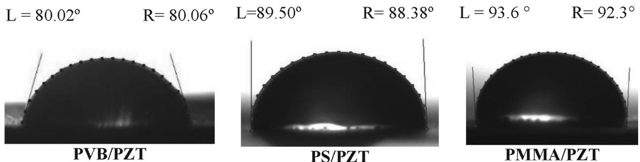
Figure 5: Water-drop profile on the PZT composite material surface polynomial fit
