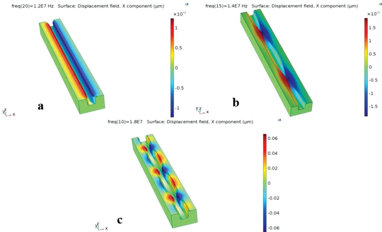
**Figure 10:** a) Surface deformation of microchannel periodically excited at 12 MHz frequency, b) microchannel periodically excited at 14 MHz and c) microchannel periodically excited at 18 MHz frequency with visualized X component of the displacement field
