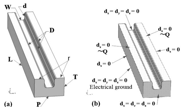
Figure 9: a) Dimensions of the finite-element model of the microchannel and b) the boundary condition of the finite-element model of the microchannel
