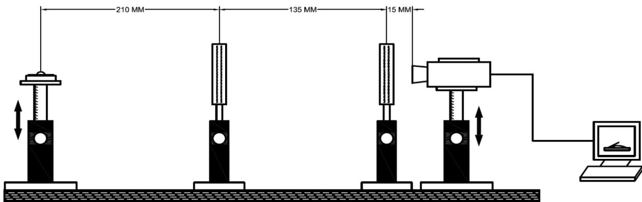
Figure 3: Illustration of the critical distance between the important parts (camera, lens, and specimen with a drop)
