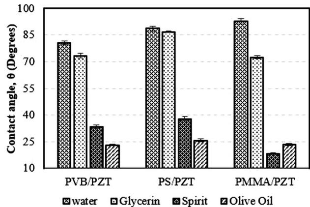
Figure 6: Mean contact angle with different liquids on three different PZT composite polymer surfaces
