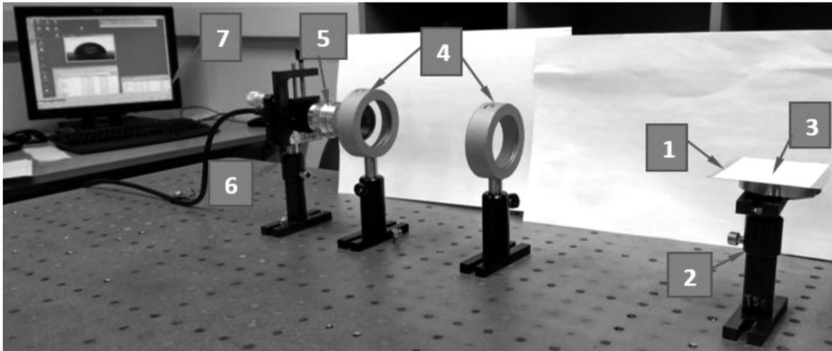
Figure 2: Experimental setup for contact-angle measurement
