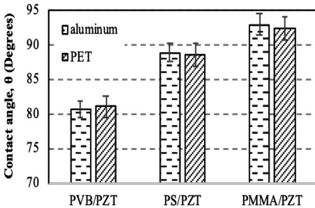
Figure 7: Comparison of WCA on Different base material
