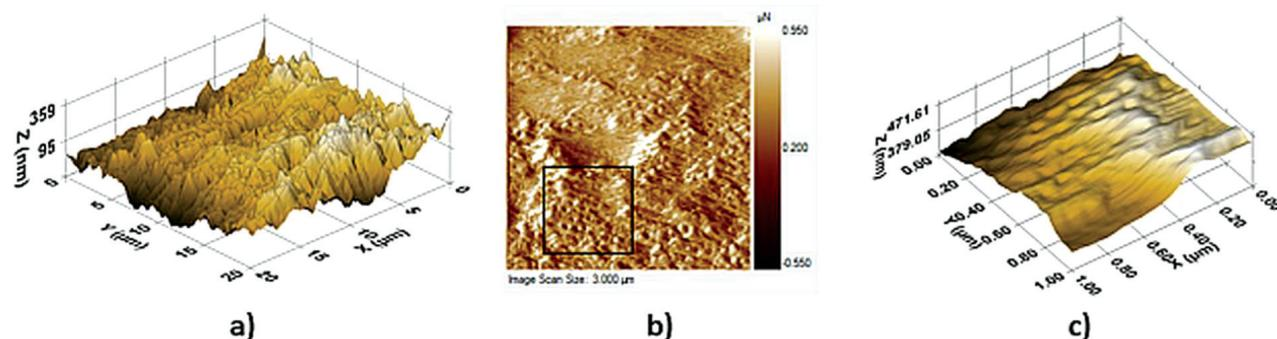
**Figure 4:** *In-situ* SPM images: a) 3D topography of titanium foil, b) map of gradients of forces obtained from TiO<sub>2</sub> NTs with 100 nm in diameter sample and c) 3D topography of the area demarcated by a black square in the picture from b)
