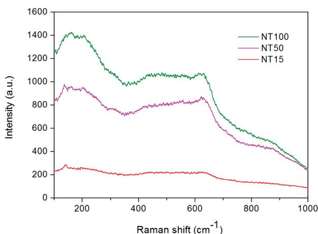
**Figure 5:** Raman spectra of TiO<sub>2</sub> NTs with various diameters. T=Ti substrate
