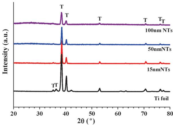
Figure 6: X-ray diffraction (XRD) patterns of Ti substrate and TiO<sub>2</sub> NTs with various diameters (T=Ti substrate)
