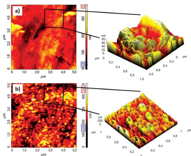
**Figure 3:** AFM images of: a) Ti foil, b) TiO<sub>2</sub> NTs with 100 nm in diameter. Zoomed region (along vertical z-direction) shows further topological details
