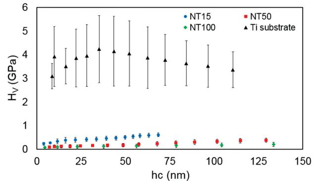
Figure 9: Depth profiles of calculated Vickers hardness. The Vickers hardness was calculated from the measured apparent indentation hardness *H<sub>v</sub>* (GPa) = 0.92666\**HIT*
