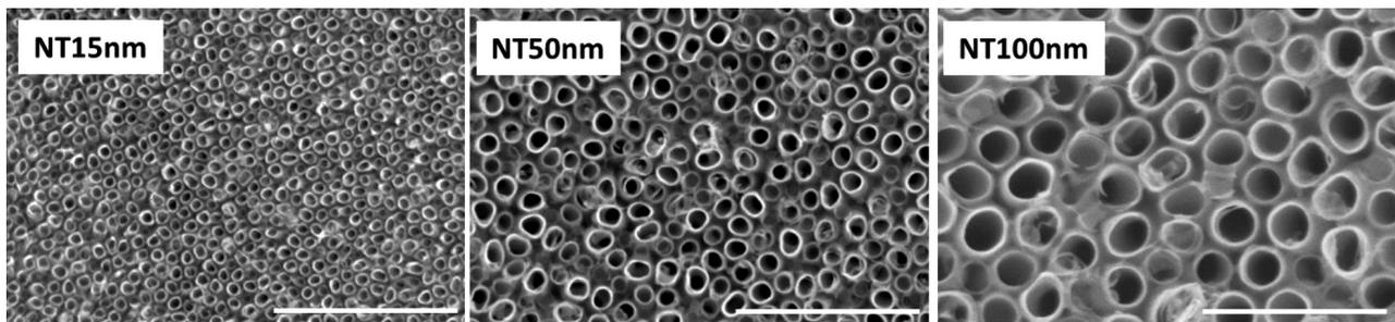
**Figure 2:** SEM images of the top surface of TiO<sub>2</sub> NTs (size of the scale bar=500 nm)
