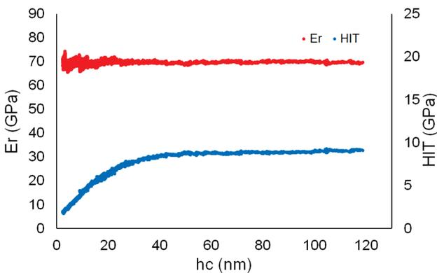
Figure 7: Calibration values of *E* and *H* vs. contact depth on fused quartz sample
