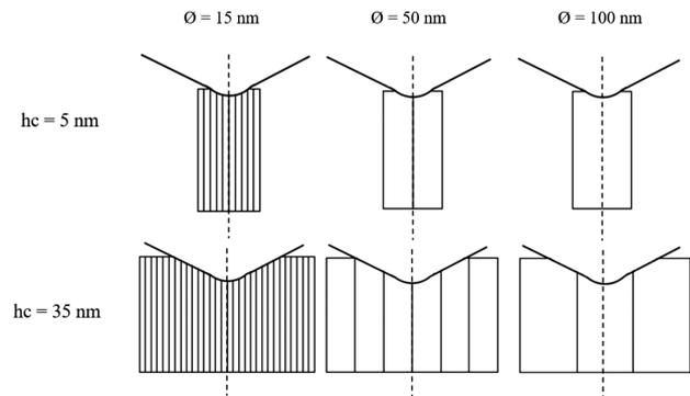
**Figure 1:** Schematic representation of contacts of the Berkovich indenter and TiO<sub>2</sub> NTs in the nano-indentation test
