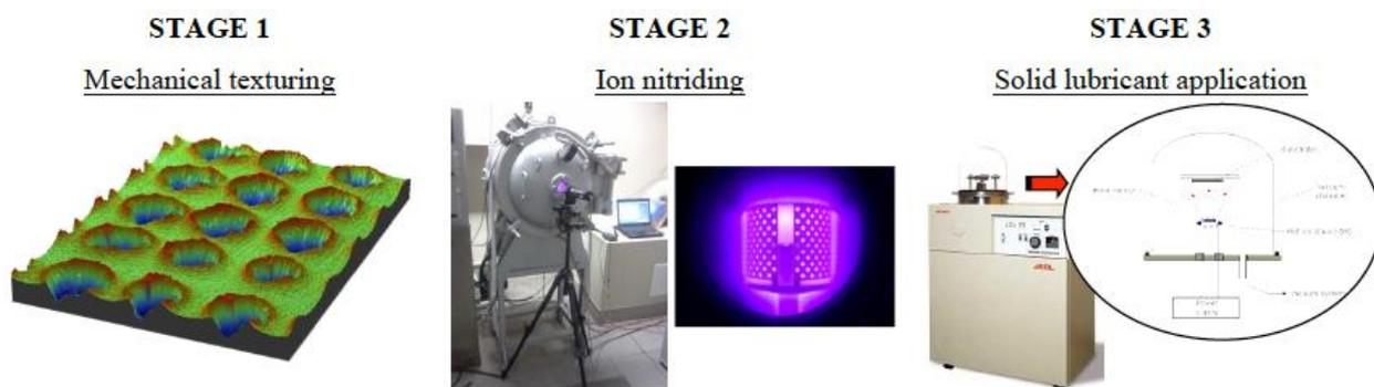
Fig.1. Multiplex surface treatment applied for Ti6Al4V
