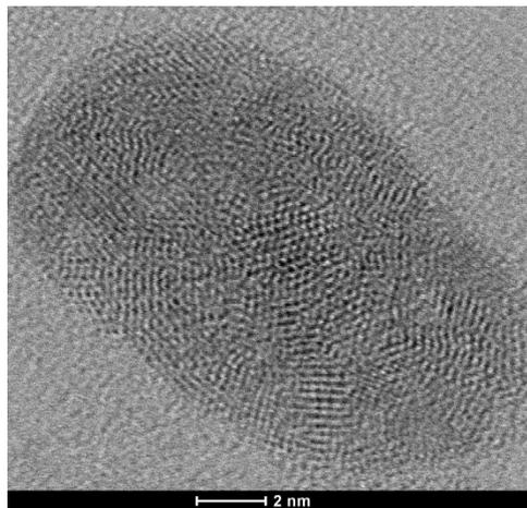
Fig. 1. BF image of nanometric intermetallic precipitate in aluminum matrix
