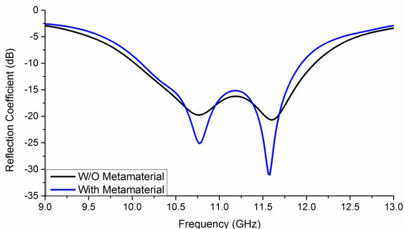
Fig. 1. Reflection coefficient of proposed antenna.
