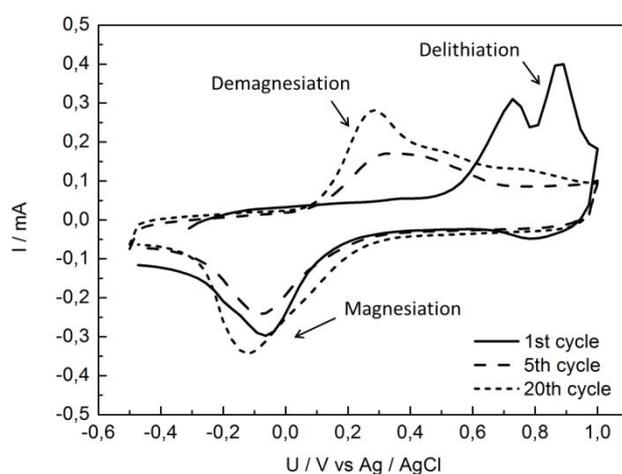
Figure 1: Cyclic voltammogram of  $\text{LiMn}_2\text{O}_4$  in  $0,1 \text{ M Mg}(\text{NO}_3)_2(\text{aq})$  in potential window between  $-0,5$  and  $1,0 \text{ V vs Ag / AgCl}$  at sweep rate  $5 \text{ mV s}^{-1}$ . Peaks indicating magnesium intercalation are visible.
