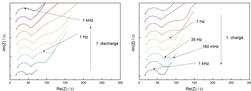
Figure 1: Change in impedance spectra during first discharge and charge (ionic liquid based electrolyte)
