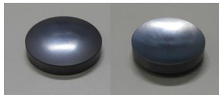
Fig.2 Si lens formed at 800  $^{\circ}\text{C}$  with SPS
