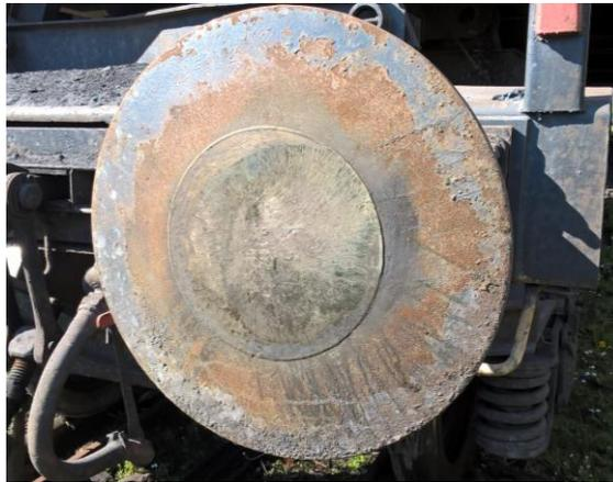
Fig. 1 The railway buffer head covered with bronze layer
