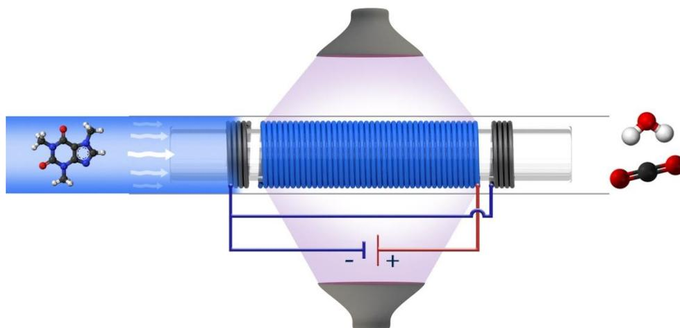
Figure 1: Schematic presentation of the caffeine degradation inside a coil-type photoelectrocatalytic microreactor.
