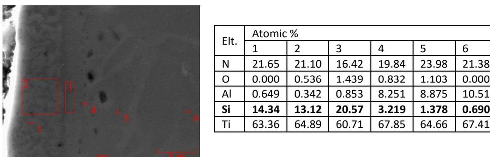
Fig.1. SEM image and EDS analysis of Ti6Al4V alloy pack siliconized at 1000°C for 10 hours.
