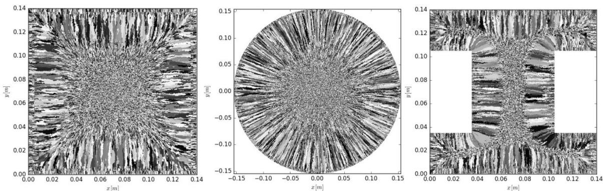
**Figure 1:** Final microstructure in the CC of steel for different cross sections of billet.
