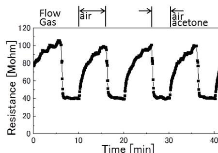
Fig. 2 Repetitive response to 500 ppm acetone gas at 300 °C
