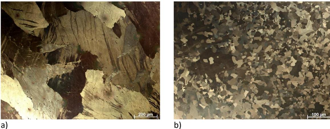
Figure 1. Microstructure of the AlMg5 aluminium alloy subjected to the a) 2 ECAP pass route Bc, b) 2 ECAP pass route Bc and annealed at 350 °C for 30 min
