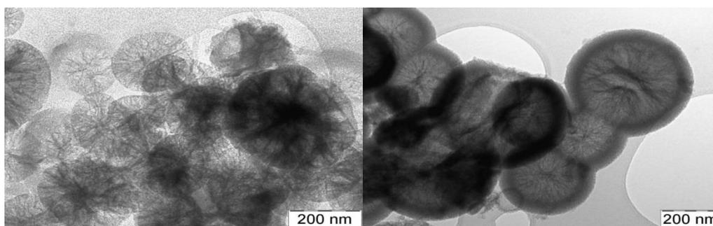
Figure 1: TEM pictures of pristine (left) and surface modified (right) silica particles.
