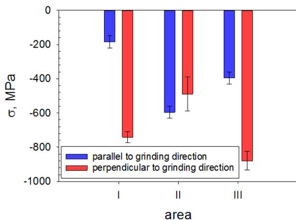
Fig. 1 RS of coarse-grained surface.
