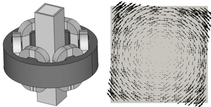
**Figure 1:** A sample geometry of the M-EMS (left) and the time averaged force on the horizontal plane in the mould (right).
