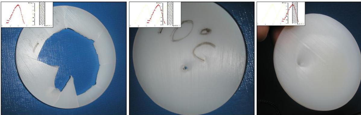
Figure 1: High-rate impact characterization, examples of PA6 impact behavior at different temperatures
