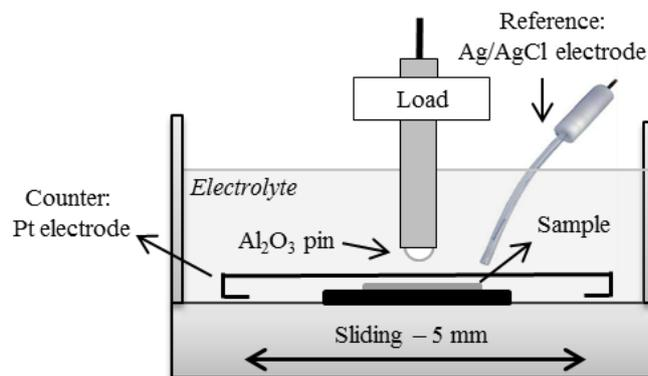
Figure: Set-up of tribocorrosion experiment
