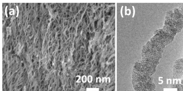
Fig. 1 (a) SEM image and (b) TEM image of SiO<sub>2</sub>/SnO<sub>2</sub> nanofibers
